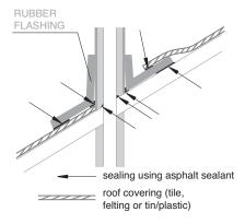
Install the ventilation pipe and seal the passage through the exterior roof using asphalt sealant to prevent leaks.
